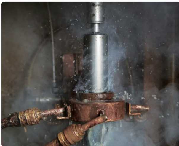
Superior durability comes from induction hardening of the cylinder's ram shaft.
