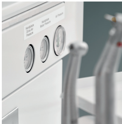
Air and water pressure gauges
