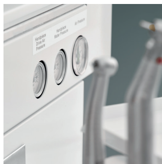
Air and water pressure gauges
